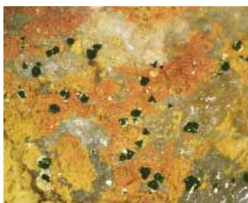
Optical microscope image of a surface coated by iron oxides and clays together with supergene gold crystals
