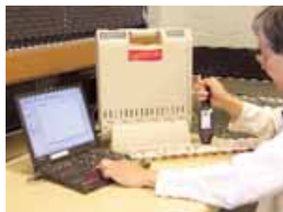
Portable ASD spectro-radiometer producing automatic mineralogical analysis from rapidly read VSWIR spectra
