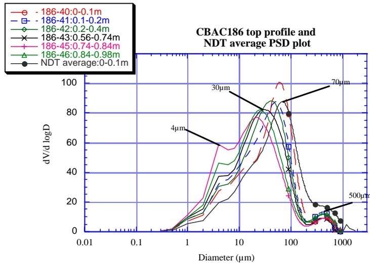
**Figure 5:** PSD plots of the alluvial CBAC186 site surface 1 m profile samples, plotted with the average NDT PSD plot.
