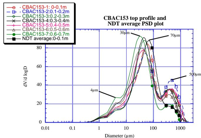
**Figure 4:** PSD plots of the colluvial CBAC153 site surface 0.7 m profile samples, plotted with the average NDT PSD plot.
