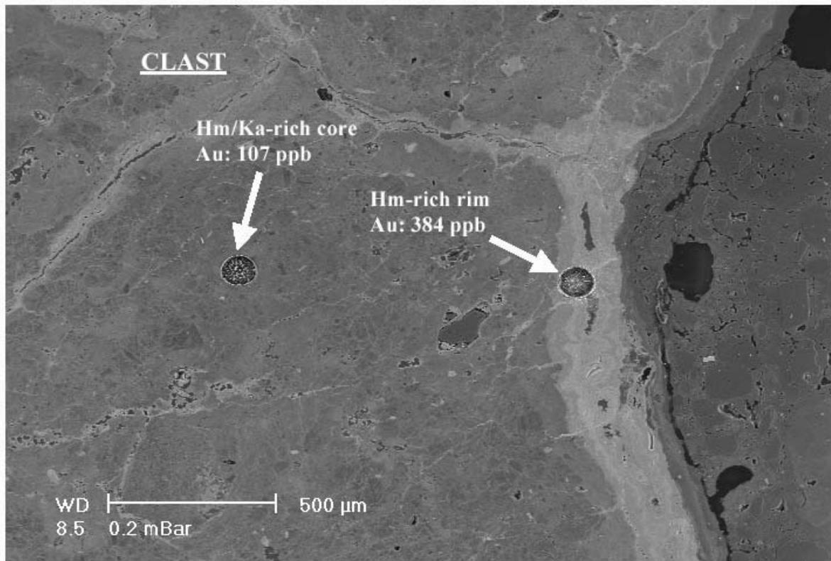
**Figure 2:** SEM (BE) image showing laser pit positions of LA-ICPMS analyses in the nodular duricrust sample (0560). Hm- hematite, Ka- kaolinite.
