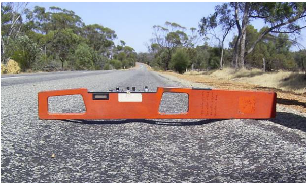
Figure 2. An EM38 meter sitting on a severely rutted rural road.
