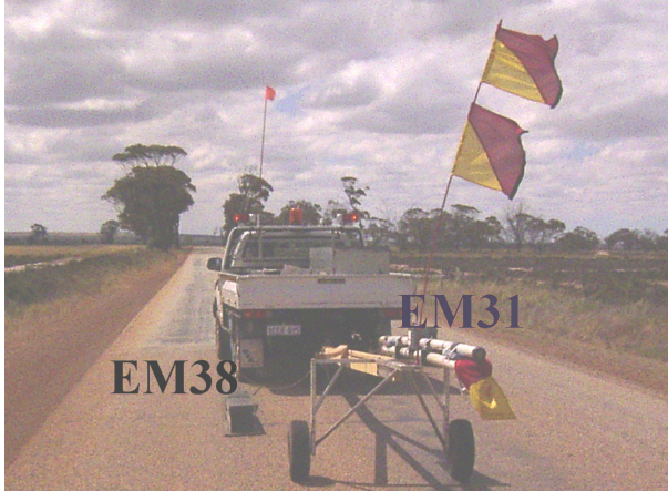
Figure 1. EM equipment towed behind a vehicle on a country road in Western Australia.
