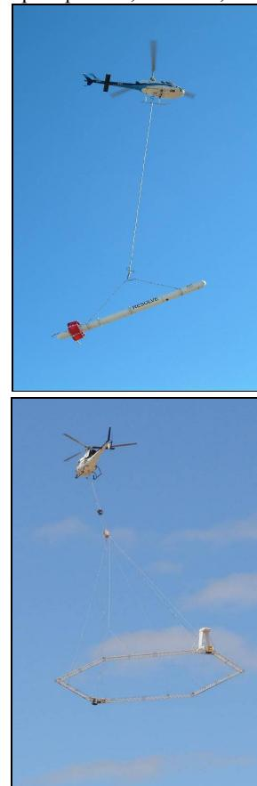
**Figure 2. The RESOLVE FDHEM (top) and SkyTEM TDHEM (bottom).**
