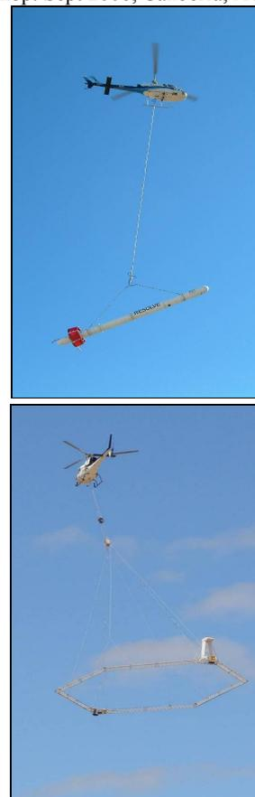
**Figure 2.** The RESOLVE FDHEM (top) and SkyTEM TDHEM (bottom).
