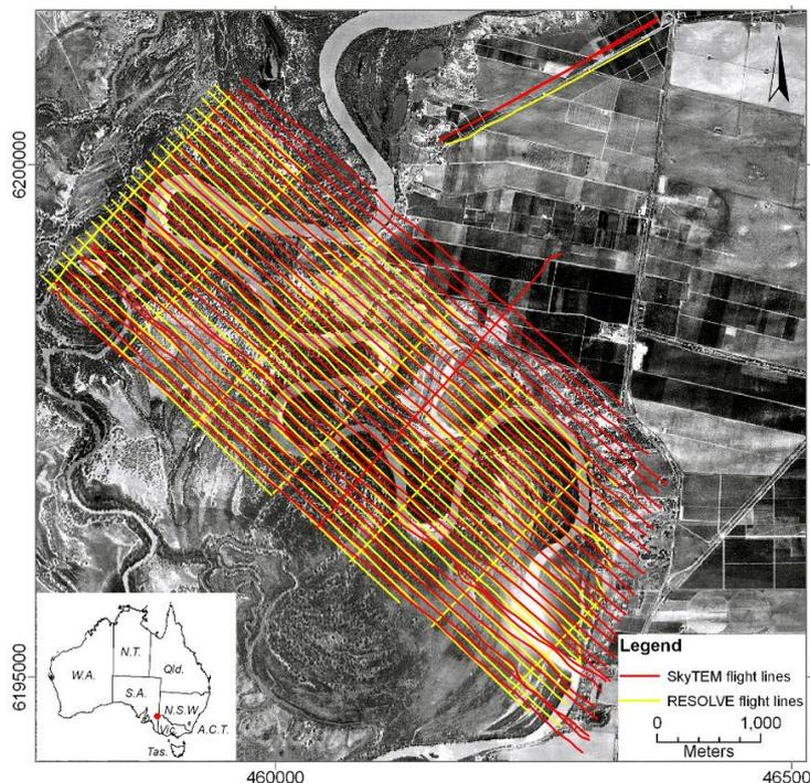
**Figure 1.** Location of the Bookpurnong Floodplain study site in South Australia. Lines for two EM systems, the RESOLVE (yellow) and SkyTEM (red) systems are shown. The survey area covers most of the Bookpurnong floodplain and parts of the adjacent highlands where irrigated agriculture has been developed. Near-coincident calibration lines (2 for SkyTEM and 1 for RESOLVE) were acquired along Nitschke Road, orientated NE-SW north-east of the survey area.
